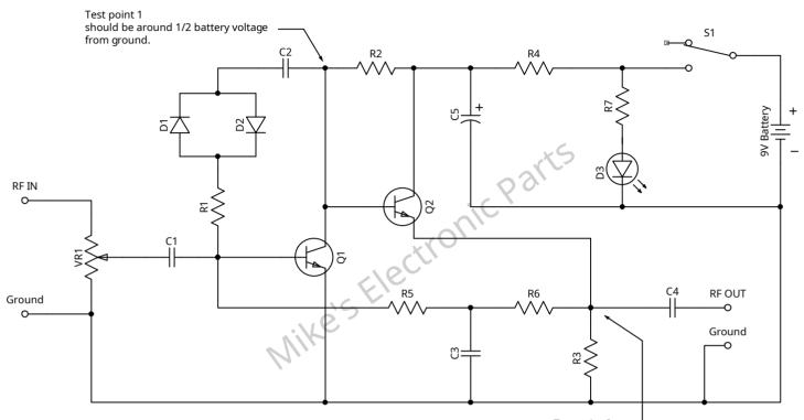
Test point 2 should be around 0.6 volts lower than test point 1
