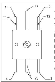
This is the pin out for the Dual 0-335pf - 0-20pf Poly Variable Capacitor. The Drawing View is looking down at the top side with the pins oriented as shown. Pins T1 and T2 are on the bottom. All Pins Marked "G" are ground connections.
