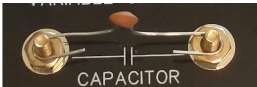
Figure 1 Wire around screws
