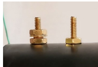
Figure 8 Coil wire, washer and nut
